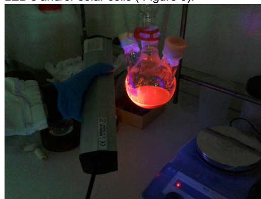
Figure 3. Luminescent perovskite quantum dots upon excitation using UV light.
